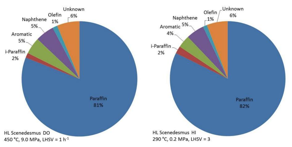
Liquid phase has same composition before and after isomerization step
