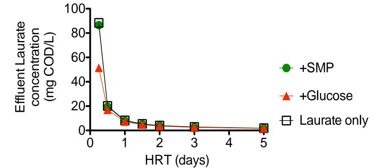
Modeled effluent laurate concentrations for a PBR with an initial laurate concentration of 100 mg COD/L and with either 10 mg COD/L SMP or 10 mg COD/L glucose.
