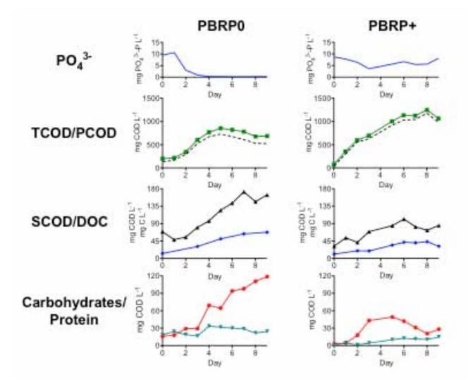
Depleting phosphate (PBR0) shows dramatic loss of biomass growth (PCOD) and increase of SMP (SCOD) and carbohydrates.
