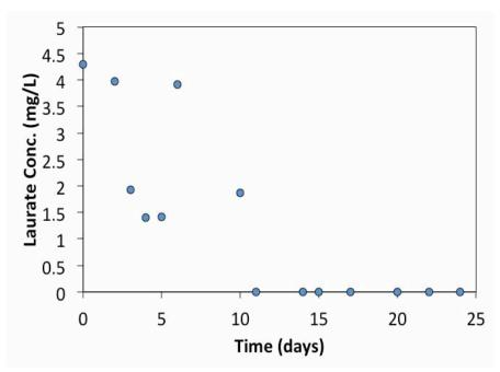
Laurate concentration in the effluent for the PBR with the resin and GAC columns throughout sequencing-batch operation.
