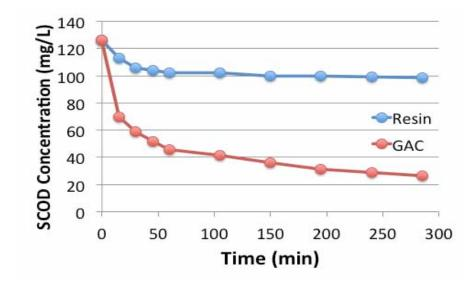
Kinetics of SMP adsorption from membrane permeate of wild-type *Synechocystis* on MP-64 resin and F-300 GAC.
