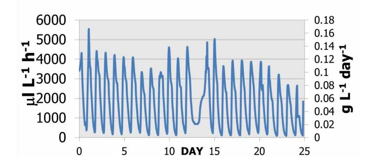
Longevity of light-dependent ethylene production in a 2L photobioreactor operated under 12h/12h diurnal cycles. Longest test was 72 days under continuous light where productivity was maintained.
